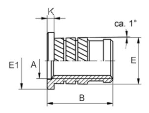
Female thread A = M3Flange diameter E1 = 5.6Flange heigth = 0.6Length B = 5.9Min distance to edge = 2.0 Outer diameter E = 4.20
